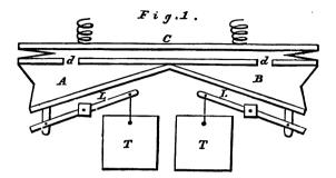
Fig. 1 shows the pressure-bellows, A and B, in a state of rest (these are sometimes called feeders, as they supply the wind); T T are the Treadles or Foot-boards; L L the levers belonging to the Treadles; d d openings for the passage of the air from the Feeders into the Reservoir.
